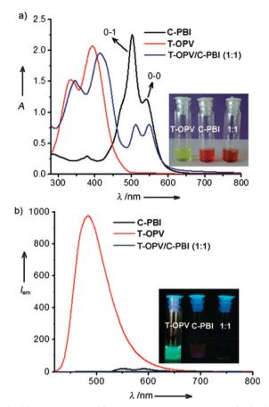
Fig. 6 (a) Absorption and (b) emission spectra for the donor (T-OPV) and acceptor (C-PBI) and the 1:1 mixture showing a strong charge transfer band and lack of fluorescence. Figure reproduced from ref. 80 with permission from John Wiley and Sons.
