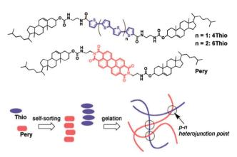
Fig. 3 The structures of Thio and Pery LMWG and a cartoon representation of the self-sorted network formed, which leads to p-n heterojunction points. Reprinted with permission from ref. 39. Copyright 2008 American Chemical Society.
