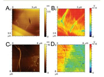
Fig. 6 AFM and EFM images. Topography of (A) A $\beta$  (16–23) and (C) F-A $\beta$  (16–23); electrostatic force map of (B) A $\beta$  (16–23) and (D) F-A $\beta$  (16–23). Peptides were 0.5 mg ml $^{-1}$  solutions in 10 mM phosphate buffer at pH 7.4 diluted 100-fold in ultrapure water and cast on Au-coated Si wafer.
