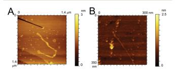
Fig. 4 AFM images of (A) A $\beta$  (16–23) and (B) F-A $\beta$  (16–23), 0.5 mg ml $^{-1}$  in 10 mM phosphate buffer at pH 7.4 diluted 100-fold in ultrapure water cast and imaged on HOPG.
