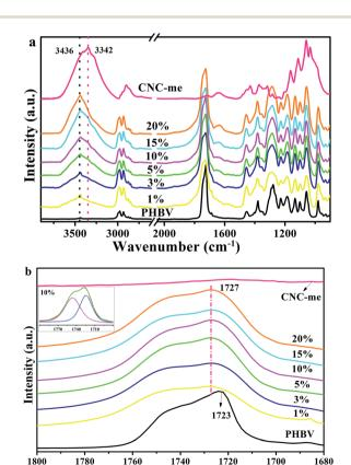
Fig. 4 FT-IR spectra (a) and carbonyl stretching region ( $v_{C=O}$ ) in the infrared spectra (b) for neat PHBV, CNC-me and the nanocomposites with various CNC-me concentrations and peak deconvolution for the nanocomposites with 10 wt% CNC-me (insert).
