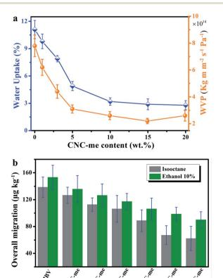
Fig. 9 Water uptake and water vapour permeability (WVP) (a), and overall migration data in ethanol 10% (v/v) and isooctane (b) as a function of CNC-me concentrations for neat PHBV and the nanocomposites.
