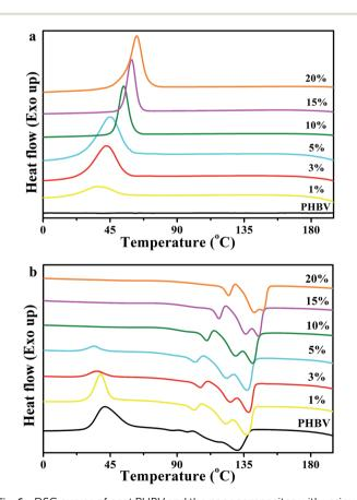
Fig. 6 DSC curves of neat PHBV and the nanocomposites with various CNC-me concentrations. (a) the first cooling trace; (b) the second heating trace.
