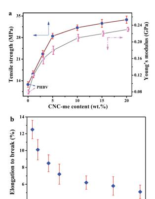
Fig. 7 Tensile strength and Young's modulus (a), and elongation to break (b) as a function of CNC-me concentrations for neat PHBV and the nanocomposites.
