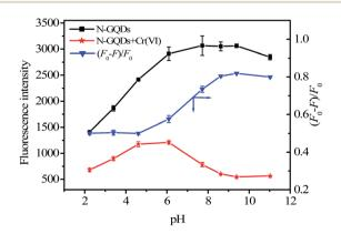
Fig. 3 FL responses of 52 mg  $L^{-1}$  N-GQDs at 430 nm in the absence (black triangle) and presence (black square) of 140  $\mu$ M Cr(vI) ions at different pH values. Relative FL intensities  $[(F_0 - F)/F_0]$  at 430 nm of solutions of N-GQDs in the presence (blue) of 140  $\mu M$  Cr(vi) ions at different pH values.
