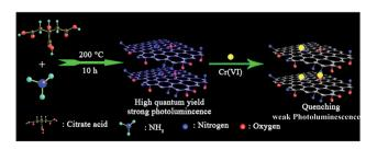
Scheme 1 Schematic diagram of fluorescent N-GQDs for  $Cr(v_i)$  sensing.
