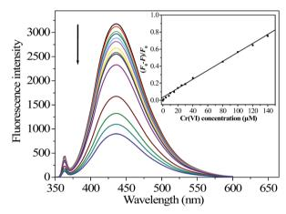
Fig. 5 FL response of 52 mg L<sup>-1</sup> N-GQDs upon addition of different concentrations of Cr(vi) ions solution. The arrows indicate the signal changes as increases in analyte concentrations (0, 1, 4, 8, 10, 15, 20, 25, 30, 40, 80, 120, and 140  $\mu$ M). Inset: plot of the values of  $(F_0 - F)/F_0$  at 430 nm versus the concentrations of Cr(vi). The error bars denote standard deviations based on three independent measurements.
