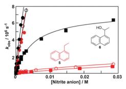
Fig. 6 Quenching plots for the guenching of the triplet excited states of 1-ethylnaphthalene (5, red) and 1-naphthyl-1-ethanol (6, black) by nitrite anions in water (solid circles), in the presence of 10 mM (open circles) and 40 mM (solid squares) sodium cholate. (Adapted with permission from C. Bohne, Langmuir, 2006, 22, 9100-9111. Copyright 2006 American Chemical Society.)
