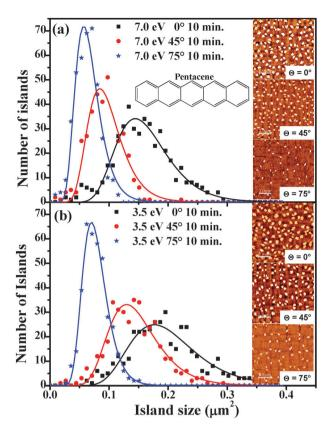
Fig. 1 Island size distribution in a pentacene sub-monolayer grown on  $\mathrm{SiO}_{\mathrm{X}}$  after 10 min of exposure to a supersonic beam of molecules with a kinetic energy of 7.0 eV (a) and 3.5 eV (b) at incidence angles  $\theta$  = 0, 45° and 75° with respect to the surface normal. The insets show the typical island morphology as a function of incident angle  $\theta$ . In (a) the scheme of the pentacene molecule is also shown.
