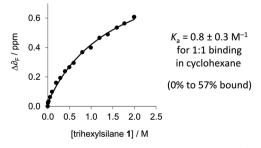
Fig. 5 1:1 binding data for the titration of trihexylsilane (1) against a constant concentration of perfluoro-tert-butanol (2) (1 mM in cyclohexane at 298 K). Additional data are presented in the ESI.‡
