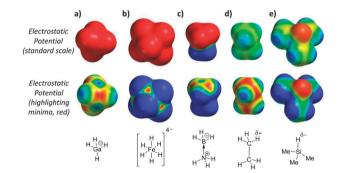
Fig. 2 Electrostatic surface potentials (ESPs) of representative dihydrogen bond acceptors. Electrostatic potentials on the top row are scaled using a standard scale from  $-50~\rm kJ~mol^{-1}$  (red) to  $+50~\rm kJ~mol^{-1}$  (blue), while those on the bottom row are scaled to highlight the ESP minimum (ESP<sub>min</sub>, red) to ESP<sub>min</sub>  $+50~\rm kJ~mol^{-1}$  (blue). Minimised geometries and ESPs were calculated using B3LYP/LACVP.
