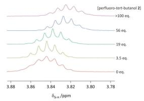
**Fig. 4** Upfield  ${}^{1}$ H-NMR chemical shift seen for the Si-H in trihexylsilane (20 mM) in cyclohexane- $d_{12}$  upon increasing the concentration of perfluoro-tert-butanol at 298 K.
