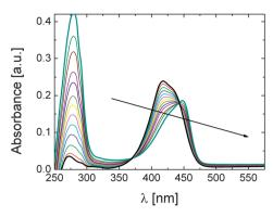
**Fig. 4** Absorbance spectra of **P1** solution in PBS  $(0.005 \text{ g L}^{-1})$  at 15 °C containing varying amounts of the antibody [from 6.7 nM to 660 nM]. The direction of the arrow shows the increase in antibody concentration.
