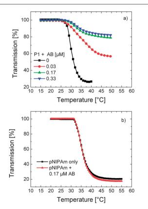
**Fig. 5** Temperature–transmission profiles of (a) **P1** solution in PBS (0.1 g  $L^{-1}$ ) containing varying amounts of the antibody (AB) (0, 0.03, 0.17, and 0.33  $\mu$ M) and (b) a solution of unlabelled pNIPAm in PBS (0.01 g  $L^{-1}$ ) in the presence (red triangles) and absence of the antibody (0.17  $\mu$ M) (black squares).
