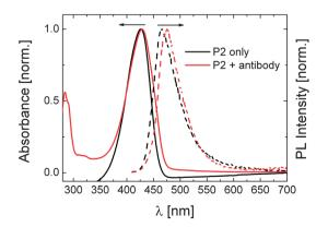
**Fig. 9** Normalised absorbance (solid lines) and PL (dashed lines) spectra of the aqueous solution of **P2** (0.01 g  $L^{-1}$ ) in the presence and absence of 0.17  $\mu$ M of antibody at 20 °C. The absolute PL spectra are given in Fig. S10.†
