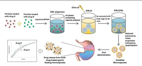
Scheme 1 Schematic illustration of the encapsulation procedure for the preparation of floating microcapsules and the release of multiple drugs within the gastric region
