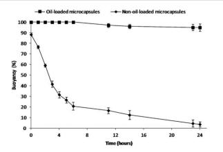
**Fig. 2** Percent buoyancy *vs.* time profiles of the present floating formulation compared with the non-oil-loaded microcapsules.
