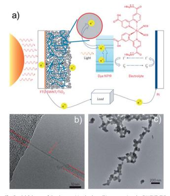
Fig. 2 (a) Scheme of the dye-sensitized solar cell incorporating the SWCNT-TiO<sub>2</sub> complex, (b) HRTEM image of a virus-SWCNT complex. A SWCNT is indicated by an arrow and the virus is indicated by dashed lines. (c) TEM micrograph of TiO<sub>2</sub> biomineralized on the virus-SWCNT complex. Adapted from Dang et al.,27 with permission from Nature Publishing Group.
