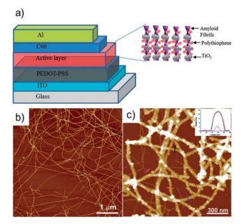
Fig. 3 (a) Schematic diagram of the hybrid photovoltaic device composed of the TiO<sub>2</sub>-hybrid nanowires blended with polythiophene. (b) Atomic force microscope (AFM) image of the β-lactoglobulin AF showing long linear semiflexible structures. (c) AFM image of TiO<sub>2</sub> decorating the surface of the AFs. Reprinted with permission from Bolisetty et al.,29 ©(2012) John Wiley & Sons.
