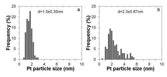
Fig. 3 Particle size distribution from image analysis of TEM pictures for Pt nanoclusters deposited onto the TiO2 support after 1 ALD cycle (a) and after 5 ALD cycles (b).
