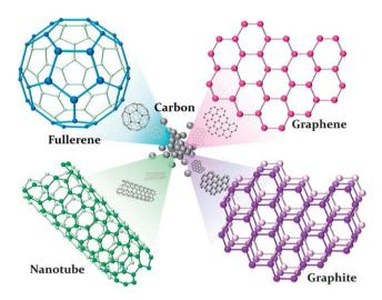
Fig. 2 Carbon allotropes in different structures.
