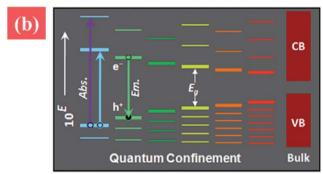
**Fig. 3** (a) Photographs and photoluminescence spectra of quantum dots with various particle sizes, and (b) qualitative alternatives of quantum dots with increased particle size. Reprinted from ref. 12 with permission. Copyright (2011) John Wiley & Sons.
