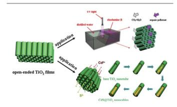
Fig. 14 Schematic of applications of free-standing open-ended TiO<sub>2</sub> nanotube membranes (reprinted with permission from ref. 113, copyright 2012 Elsevier).
