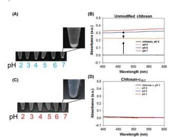
**Fig. 2** (A) Photographs of the chemically unmodified chitosan solutions at pH values ranging from 2 to 7 and (B) the UV-vis absorbance spectra of the chitosan at pH 2 (green), 4 (orange), 6 (blue), and 7 (red). The arrows indicate the baseline upshifts as pH increases, as an indication of the insolubility of chitosan. (C) Photographs of the chitosan-c solutions at pH ranging from 2 to 7, and (D) the UV-vis absorbance of chitosan-c at pH 2 (green), 4 (orange), 6 (blue), and 7 (red).
