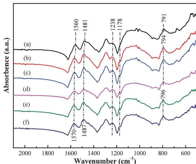
**Fig. 4** FT-IR spectra of the PNCs (a) before and after treatment with Cr(VI) solution with an initial Cr(VI) concentration of (b) 1.0, (c) 2.0, (d) 3.0, (e) 4.0 and (f) 5.0 mg L<sup>-1</sup>.
