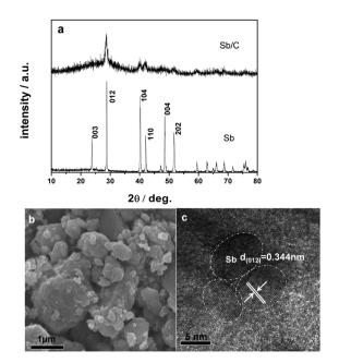
**Fig. 1** (a) X-ray diffraction patterns of the Sb/C nanocomposite and metallic Sb. (b and c) SEM and HRTEM images of the Sb/C nanocomposite.
