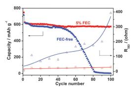
Fig. 3 Changes of the cycling capacities and SEI film resistances of the Sb/C anodes in the 1.0 mol L<sup>-1</sup> NaPF<sub>6</sub> + EC-DEC electrolyte with (red  $\blacksquare \square$ ) and without (blue  $\blacktriangle \triangle$ ) the addition of 5% FEC additive.
