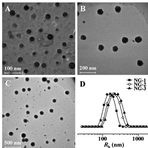
**Fig. 3** TEM micrographs of NG-1 (A), NG-2 (B) and NG-3 (C), and hydrodynamic radii ( $R_h$ ) of NGs (D).
