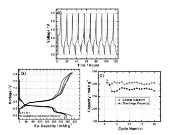
Fig. 3 (a) Voltage vs. time (b) voltage vs. sp. capacity and (c) cycle life plot of Al-ion battery containing aluminium anode,  $V_2O_5$  nano-wire cathode in ionic liquid under the potential window 2.5–0.02 V and at a constant current drain of 125 mA  $\rm g^{-1}$ .
