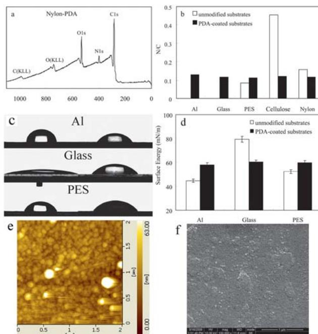
**Fig. 2** (a) XPS spectra of PDA-coated nylon; (b) the N/C molar ratio; (c) water contact angles of the PDA-coated substrates; (d) the surface energy of the PDA-coated substrates; (e) AFM and (f) FSEM images of the surface morphology of the PDA-coated glass.
