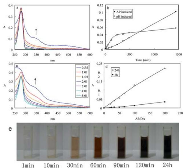
**Fig. 1** (a) UV-vis spectra of DA during the AP-mediated oxidation reaction. (b) Absorption intensity at 350 nm of DA by both oxidant-induced and pH-induced. (c) UV-vis spectra of DA after 24 h running time by mixed with different amount of AP. (d) Absorption intensity at 350 nm of DA after 2 h and 24 h running time when mixed with different amounts of AP. (e) Colour change of DA with the running time.
