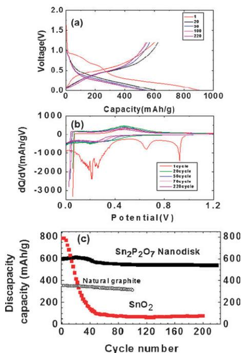
**Fig. 2** (a) Voltage profiles of the quenched nanodisks in a coin-type half cell between 0 and 1.2 V at 0.5 C rate ( $= 350 \text{ mA g}^{-1}$ ) after 1, 20, 50, 100, 220 cycles. (b) Differential curves of (a). (c) Discharge capacity (after lithium removal) vs. cycle number in nanodisk. References are natural graphite and  $\text{SnO}_2$  nanoparticles.
