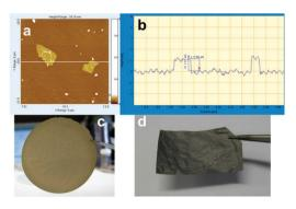
Fig. 1 (a) and (b) AFM scan of two graphene oxide sheets, showing a single layer height of about 1 nm and about  $1 \times 1$  µm wide (also determined by DLS, Fig. S3 (ESI†)). (c) Si-graphene oxide (SGO) composite paper. (d) Si-graphene (SG) composite paper obtained by reduction of SGO.
