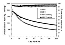
Fig. 4 Delithiation capacities and coulomb efficiencies of SG samples reduced at 550 or 850 °C, using a constant current-constant voltage (CCCV) method  $(1.5-0.020 \text{ V}, 1000-50 \text{ mA g}^{-1})$ .
