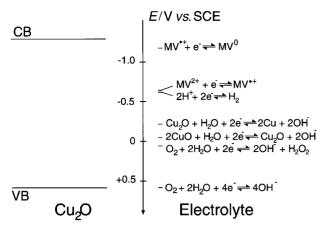
Fig. 2 Overview of the redox potentials of the relevant reactions with respect to the estimated position of the Cu<sub>2</sub>O band edges.
