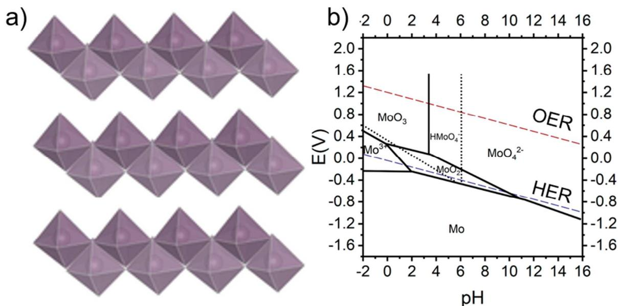
**Figure 8.** MoO<sub>3</sub> structure and solubility. a) Structure of  $\alpha$ -MoO<sub>3</sub>. Reproduced with permission from Ref. 92. Copyright 2017 John Wiley and Sons. b) Pourbaix diagram of MoO<sub>3</sub> in water: MoO<sub>3</sub> is thermodynamically stable at positive potentials and low pH electrolytes (adapted from Ref. 25).
