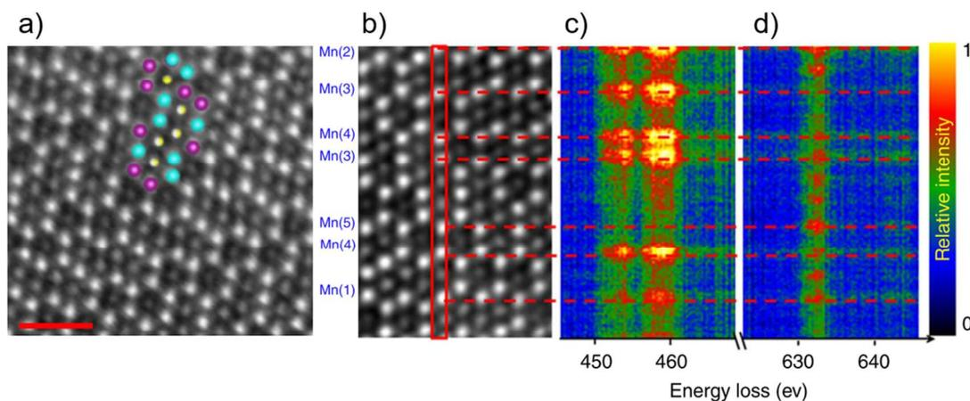
**Figure 12.** Occupation of Mn sites by Ti and Mn in  $\text{Na}_{0.44}\text{Mn}_{0.44}\text{Ti}_{0.56}\text{O}_2$ . a) & b) HAADF-STEM of the [001] zone axis, c) EELS of Ti region, and d) EELS of Mn region. These results show that Ti primarily occupies the Mn(1), (3), and (4) sites, while Mn primarily occupies the Mn(5) and Mn(2) sites. Adapted with permission from Ref. 120. Copyright 2015 Springer Nature.
