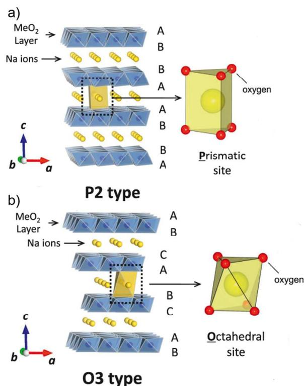
**Figure 13.** a) Structure of P2- $\text{Na}_x\text{MnO}_2$  where  $\text{Na}^+$  occupies the prismatic interlayer sites and the oxygen stacking sequence is "...ABBA...", and b) Structure of O3  $\text{Na}_x\text{MnO}_2$  where  $\text{Na}^+$
