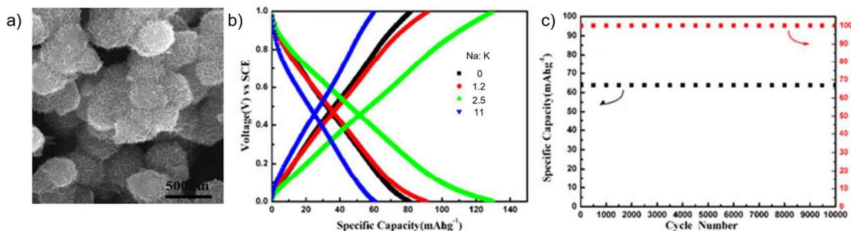
**Figure 7.** Scanning electron micrograph of the flower-like morphology of as-synthesized  $\delta$ -MnO<sub>2</sub>, b) Galvanostatic cycling of  $\delta$ -MnO<sub>2</sub> with varying ratios of Na : K at 1.5C in 1 M Na<sub>2</sub>SO<sub>4</sub>,
