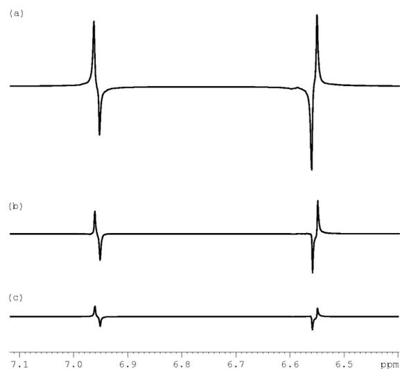
Figure 3.  $^1\text{H}$  NMR traces showing the decay in the SABRE driven singlet ( $S_0$ ) magnetisation over spin-lock times of: (a) 1 s, (b) 30 s and (c) 60 s.
