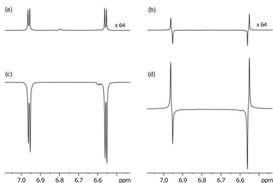
Figure 2. Plots showing the  $^1\text{H}$  NMR signals of **atz** at 400 MHz for: (a) a single shot thermally equilibrated  $^1\text{H}$  NMR spectrum, (b) a  $S_0$  derived spectrum of **atz** that is created and examined 1 s later by the method of Levitt (64 x vertical expansion relative to (d)), (c) the corresponding **3a** derived SABRE hyperpolarised **atz** spectrum and (d) the  $S_0$  state 1 s after it was created through SABRE and a spin-lock.
