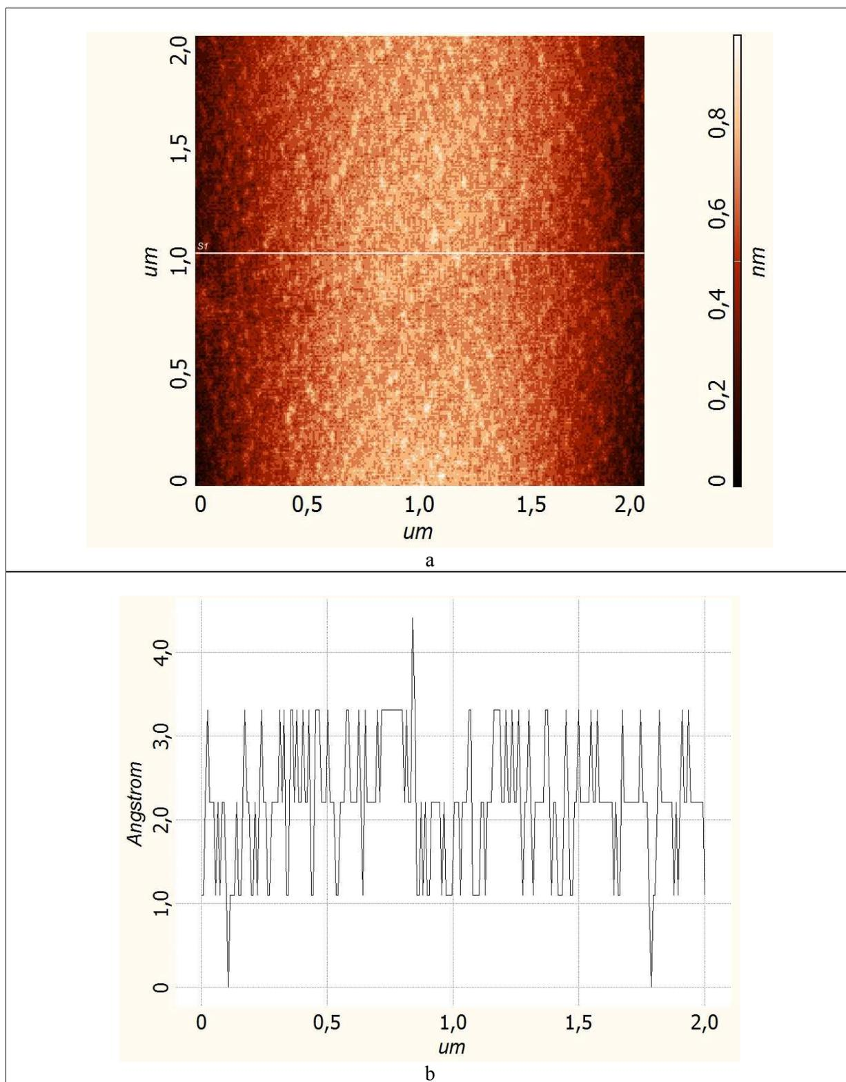
Fig. 6. An AFM pattern recorded from the  $\text{Pb}_2\text{MoO}_5(20-1)$  cleaved surface: (a) panoramic view and (b) depth profile.
