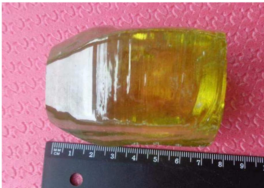
Fig. 2. A Pb<sub>2</sub>MoO<sub>5</sub> crystal grown by the LTG Cz technique. The seeding and bottom parts are cut.
