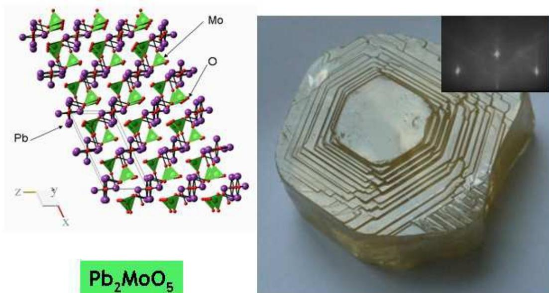
The high-quality  $\text{Pb}_2\text{MoO}_5$  crystal has been grown by LTG Cz method.
