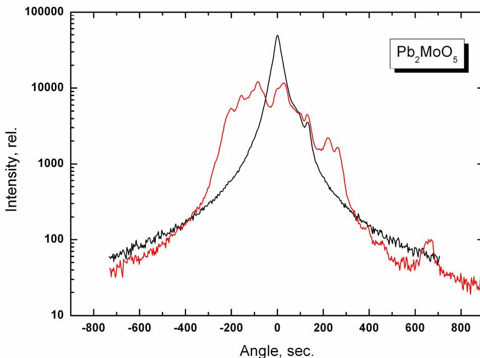
Fig. 4. Rocking curves recorded for reflex (40-2) from the (black) central and (red) peripheral parts of cleaved  $\text{Pb}_2\text{MoO}_5$ (20-1) substrate.
