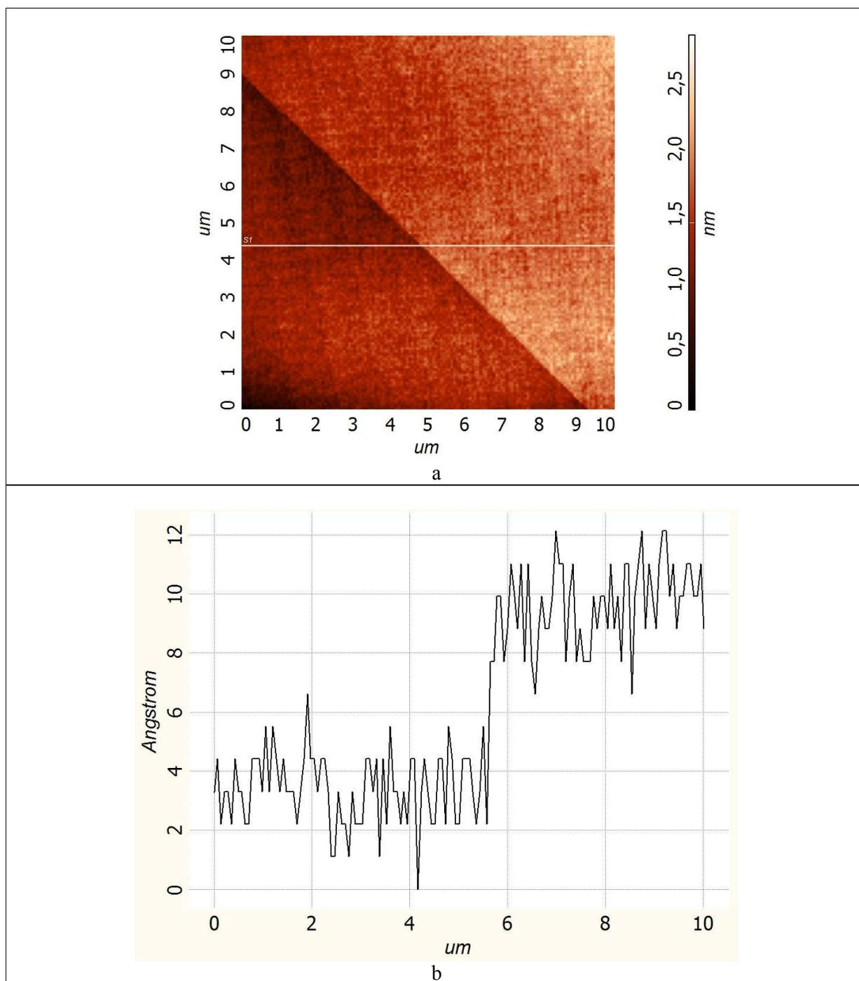
Fig. 7. An AFM pattern recorded from the region of the  $\text{Pb}_2\text{MoO}_5(20-1)$  cleaved surface with the elementary step: (a) panoramic view and (b) depth profile.
