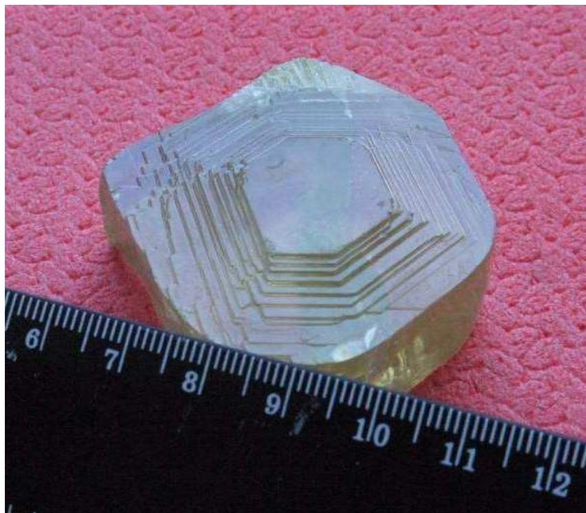
Fig. 3. Bottom part of the  $\text{Pb}_2\text{MoO}_5$  boule.
