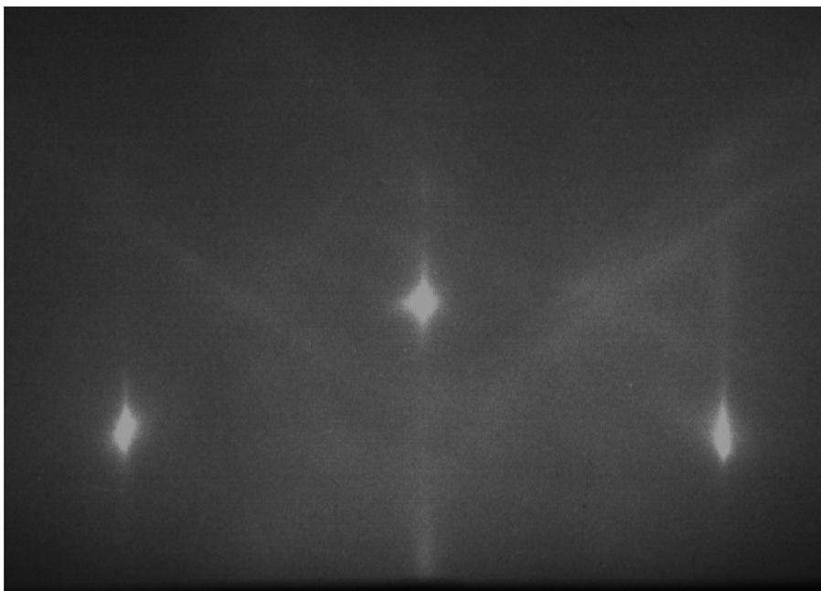
Fig. 5. A Kikuchi lines pattern recorded by RHEED for the cleaved  $\text{Pb}_2\text{MoO}_5(20-1)$  surface. The electron beam is along  $[212]$ .
