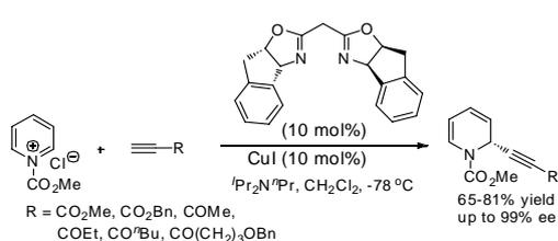
**Scheme 25** Copper-catalyzed addition of 1-alkynes to 1-acylpyridinium salts
