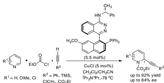
**Scheme 26** Copper-catalyzed addition of 1-alkynes to pyridines
