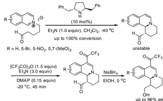
Scheme 33 Organocatalyzed annulation of alkylated isoquinolines
