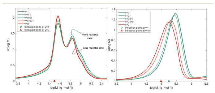
Fig. 5 Left: kMC simulation of bulk PLP of *n*BuA at a laser pulse frequency of 500 Hz and 306 K, with a variation of  $\gamma$  (eqn (2);  $\gamma = 1$  implying  $k_{\rm p,P} = k_{\rm p,e}$  and  $\gamma = 0$  implying  $k_{\rm p,P} = k_{\rm p,m}$ ). Right similar plot but at a lower laser pulse frequency of 50 Hz; on the *x*-axis the identification of the first inflection points (left coinciding; right shift). Same coloring as in Fig. 3, regarding expected behavior.
