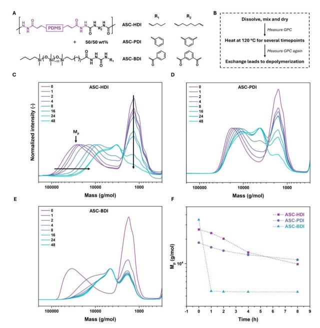
Fig. 6 (A) Chemical diagrams of ASC oligomers and mono-ASCs. (B) Workflow for measuring dissociation dynamics in bulk. Normalized mass distributions of ASC-HDI (C, RI detector), ASC-PDI (D, UV detector) and ASC-BDI (E, UV detector) mixtures at 120 °C at various times (in hours). (F) Comparison of the high molecular weight peak  $(M_p)$  over time.
