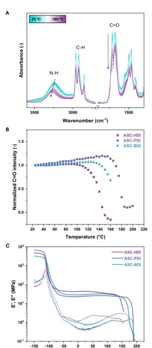
Fig. 4 (A) Variable temperature infrared spectroscopy spectra of ASC-BDI (first heating, intervals of 5 °C). (B) Intensity plot of peak maxima of the C=O stretches of pDMS-ASC materials over temperature, normalized against the intensity of the C−H stretch at 2960 cm<sup>-1</sup>. (C) Dynamic mechanical thermal analysis under extension on the ASC oligomers obtained after compression molding representing the storage (solid) and loss (dashed) moduli as a function of temperature.
