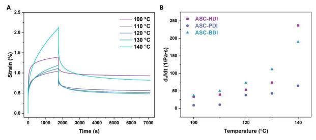
Fig. 7 (A) Creep-recovery runs of ASC-HDI at various temperatures at 20 kPa. (B) Temperature dependent slopes of the creep compliance (between 1400 and 1800 s) of ASC oligomers.
