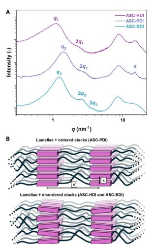
Fig. 5 (A) MAXS and WAXS 1D transmission scattering profiles of ASC-HDI, ASC-PDI and ASC-BDI. (B) Schematic representation of the ordered phase separation in the pDMS-ASC materials, highlighting the ordering within ASC stacks (purple blocks) for ASC-PDI, with indicated intermolecular spacing x.
