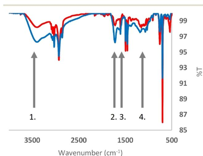
**Fig. 3** UATR-FTIR spectra for the 53 nm PS-NH<sub>2</sub> particles. Red is the control, placed in a glass Petri dish during the experiment, sample. Blue is the UV-B treated, placed in a quartz Petri dish during the experiment, sample. The grey arrows indicate some of the changes in the FTIR spectra.
