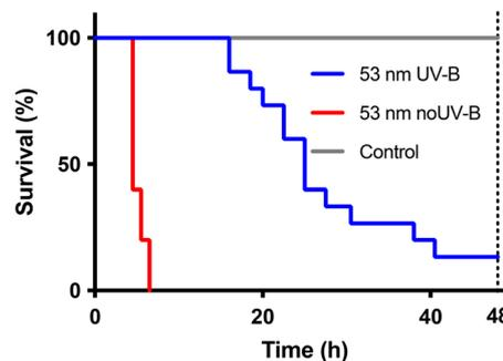
**Fig. 4** Acute toxicity test with 53 nm amine-modified polystyrene particles. Kaplan-Meier survival curves for *D. magna* exposed to UV-B exposed (blue line) and UV-B shaded (red line) nanoplastics. The grey line shows a control treatment only containing water. Total exposure time is 48 hours as highlighted by the dotted vertical line.
