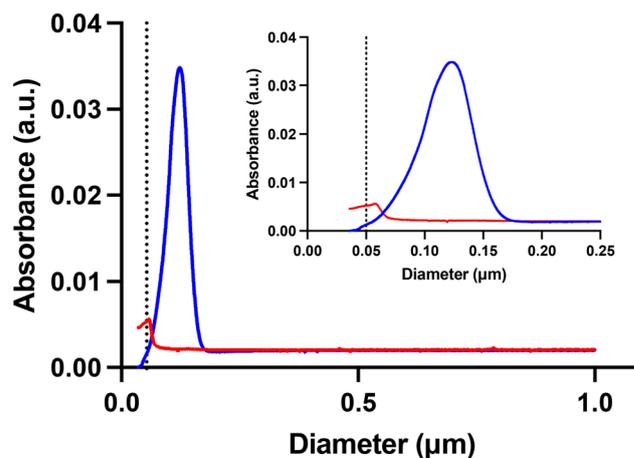
Fig. 2 The size difference measured by DSC after 100 days UV-B exposure. UV-B treated particles are in blue and untreated in red. The dotted vertical line indicates the nominal size of the starting material, i.e. 53 nm. The inset plot shows a zoom of the size range of 0–250 nm.
