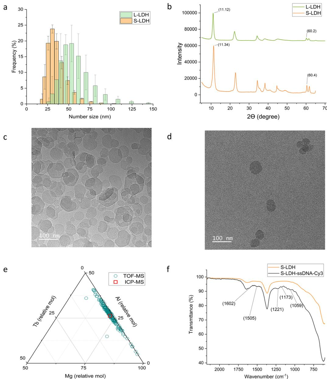
**Fig. 1** S-LDH and L-LDH characterization and surface modification. (a) Size distribution by DLS measurements. (b) XRD spectra. TEM images of (c) L-LDH and (d) S-LDH. (e) Metal ratio description of S-LDH obtained by single particle ICP-TOF-MS. The red square represents the value obtained by ICP-MS. (f) ATR spectrum of S-LDH-ssDNA-Cy3 in comparison to the S-LDH.
