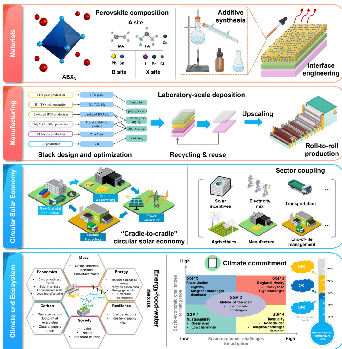
Fig. 4 Schematic of the multi-scale analytics and modeling of perovskite PV value chain. From top to bottom, four systems layers regarding different temporal and spatial scales typify the level of materials, manufacturing, circular solar economy, and climate and ecosystem, respectively. The systems scale grows from top to bottom, whereas the modeling details and resolutions increase from bottom to top.
