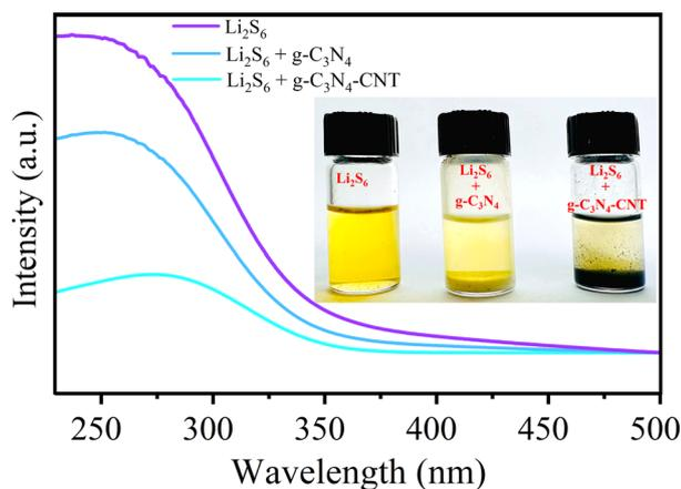
Fig. 3 UV-vis spectra for blank  $\text{Li}_2\text{S}_6$  and  $\text{Li}_2\text{S}_6$  added with CN and  $g\text{-C}_3\text{N}_4\text{-CNT}$ . The inset shows the digital picture of the effect of the active material on the adsorption of LiPSs in  $\text{Li}_2\text{S}_6$  solution.
