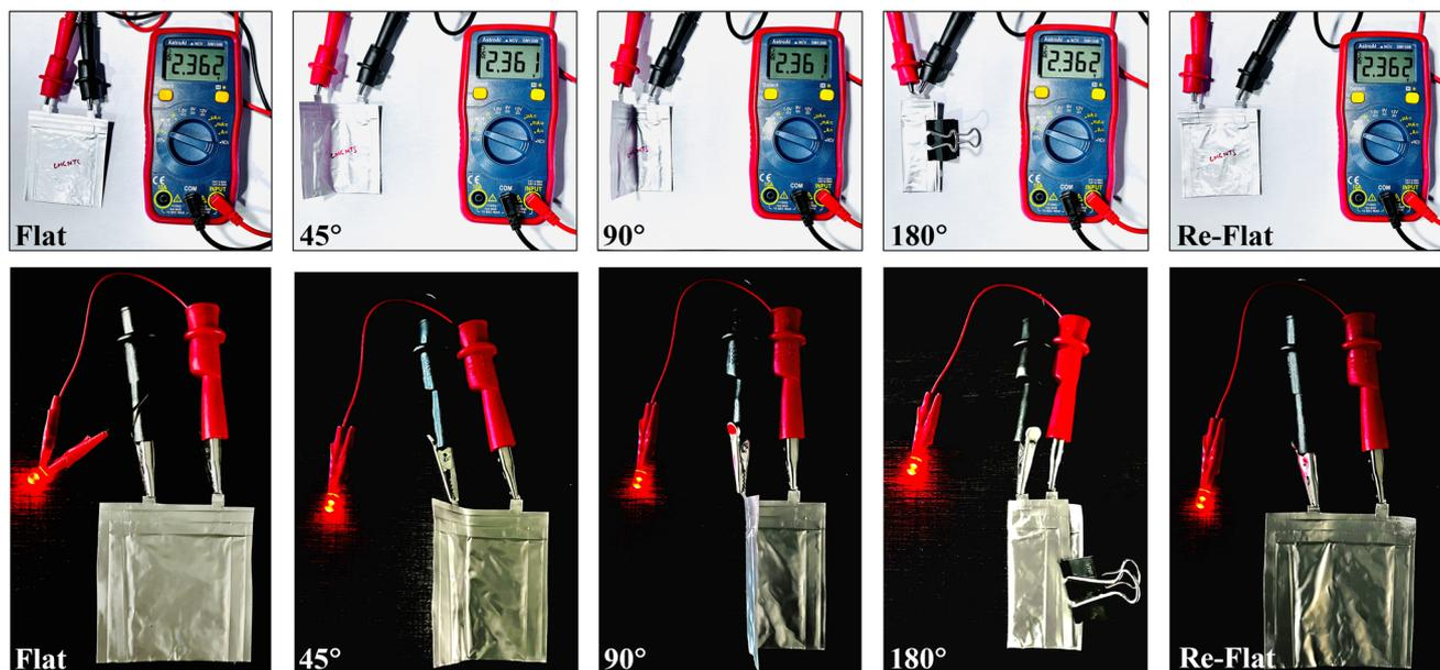
Fig. 7 Upper row: digital pictures of the OCV for the pouch cell consisting of the g-C<sub>3</sub>N<sub>4</sub>-CNT/S cathode at different folding angles and bottom row: pictures of LEDs lit up by the pouch cell at different folding angles demonstrating the excellent flexibility of the developed pouch cell.
