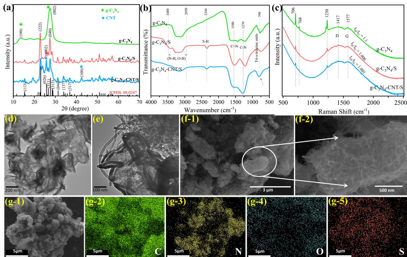
**Fig. 1** For  $g\text{-C}_3\text{N}_4$ ,  $g\text{-C}_3\text{N}_4/\text{S}$ , and  $g\text{-C}_3\text{N}_4\text{-CNT/S}$ : (a) XRD patterns, (b) FTIR spectra and (c) Raman spectra; TEM images for (d)  $g\text{-C}_3\text{N}_4$  and (e)  $g\text{-C}_3\text{N}_4\text{-CNT/S}$  materials; (f) SEM images for  $g\text{-C}_3\text{N}_4\text{-CNT/S}$ ; (g) color mapping of  $g\text{-C}_3\text{N}_4\text{-CNT/S}$  demonstrating the uniform distribution of C, N, O, and S elements.
