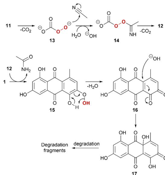
Scheme 2 Proposed mechanism for the oxidative bleaching with **12**.
