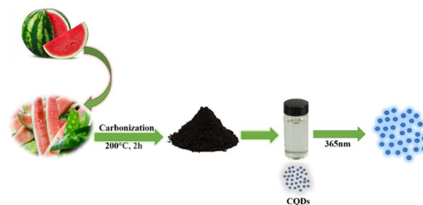
Fig. 5 A schematic illustration of the synthesis of water-soluble fluorescent CQDs from watermelon peels. 46
