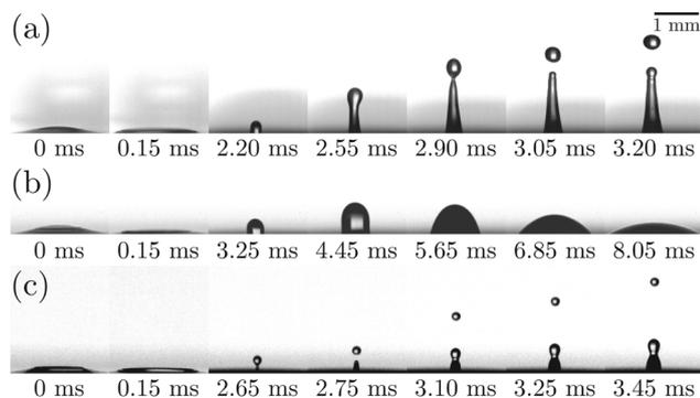
Fig. 4 High-speed images of jetting following bubble bursting at the surface of (a) pure NaCl solution, (b)  $0.05 \text{ g L}^{-1}$  BSA solution, and (c)  $0.05 \text{ g L}^{-1}$  BSA +  $0.1 \text{ g L}^{-1}$  Tween 80 solution. The aging time of the bubble is controlled to be  $t_a = 300 \text{ s}$ . The origin of time at 0 ms represents the start of bubble cap rupture.
