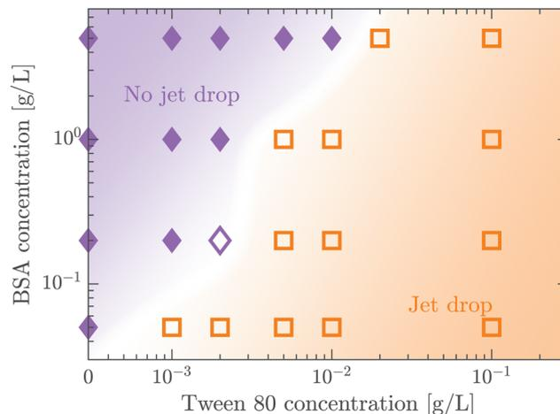
Fig. 5 Regime map of jet drop generation regarding Tween 80 and BSA concentrations. All experiments were conducted at  $t_a = 300 \text{ s}$ . The orange squares and the purple diamonds represent the experiments where jet drops are observed and not observed, respectively. The shades of colors represent corresponding regimes. The solid and empty data points represent the cases where  $E_c$  is larger and smaller than 1, respectively.
