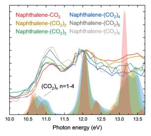
Fig. 2 Lines represent the PIE of naphthalene– $(CO_2)_p$  (p=1-6) clusters showing the three main peaks associated with the excited states of  $CO_2$ . The shaded curves are calculated absorption spectra of pure  $CO_2$  clusters (n=1-4) using TDDFT on the LC-BLYP/daug-cc-pVTZ level. Corresponding structures are displayed in ESI Fig. 2† and a full scale plot in ESI Fig. 3.† Theory is redshifted by 0.6 eV, matching the experimental band at 12 eV. Theory and experiment are normalized at 12 eV.
