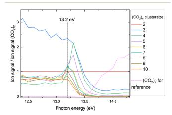
Fig. 3 PIE of pure  $CO_2$  clusters divided by  $(CO_2)_2$  as function of photon energy showing the relative abundance of higher order clusters. As a reference, the  $(CO_2)_2$  cluster PIE curve is plotted (pink, dotted line), showing that the cluster size peaks at around the appearance energy. (Note that the AE of  $(CO_2)_n$  n > 1 are very similar).
