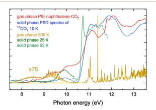
Fig. 5 Comparison of the PIE curve of naphthalene– $CO_2$  with solid phase photon-stimulated desorption (PSD) spectrum of  $^{13}CO_2$ ,  $^{20}CO_2$  gas-phase spectrum  $^{39}$  and  $CO_2$  solid phase absorption spectra.  $^{40-42}$
