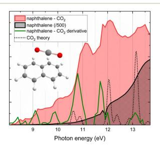
Fig. 1 PIE curves of naphthalene and naphthalene– $CO_2$  cluster showing the enhancement in ionization efficiency below the IE of  $CO_2$ . Inset shows the structure of naphthalene– $CO_2$  optimized using DFT in this work. The black dotted line corresponds to the calculated absorption spectrum of pure  $CO_2$  using TDDFT at the LC-BLYP/daug-cc-pVTZ level. The green solid line shows the derivative of the naphthalene– $CO_2$  PIE, revealing peaks that correspond to the  $CO_2$  excitations.
