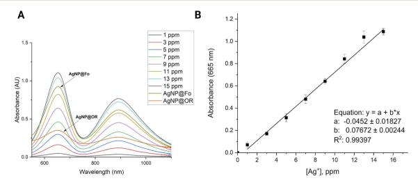
Fig. 1 Silver(i) concentration determination: (A) absorption spectra of silver(i) standards with increasing amounts of Ag<sup>+</sup> (0-15 ppm) in the presence of TMB (10 mmol  $L^{-1}$ ). (B) Linear relationship between silver ion (Ag<sup>+</sup>) concentration in (ppm) and detected absorbance at 665 nm.
