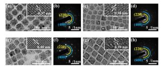
Fig. 2 TEM and HRTEM images (insets) of (a) Cs2AgInCl6, (c) 2%Bi, (e) 20%Yb, 7%Er and (g) 2%Bi@20%Yb, 7%Er NCs, and their corresponding SAED patterns (b), (d), (f) and (h). Some 'dark dots' appearing in the TEM images over the surface of the NCs are attributable to the reduction of Ag<sup>+</sup> to Ag<sup>0</sup> by Olam.<sup>21,34</sup>
