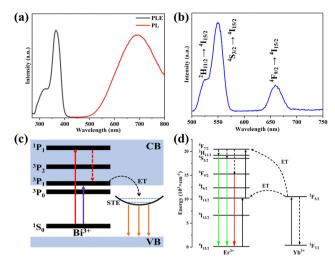
Fig. 3 PL properties of 2%Bi@20%Yb, 7%Er. (a) PL ( $\lambda_{ex}$  = 370 nm) and PLE ( $\lambda_{em}$  = 690 nm) spectra; (b) PL ( $\lambda_{ex}$  = 980 nm) spectrum; (c) schematic diagram of the energy-transfer mechanism of Bi3+ in core-shell NCs; (d) schematic diagram of the energy-transfer mechanism of Yb3+-Er3+ in core-shell NCs.
