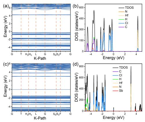
Fig. 4 DFT simulations. (a) electronic band structures and (b) density of states (DOS) of (TMA)<sub>2</sub>HfCl<sub>6</sub>; (c) electronic band structures and (d) DOS of Sb<sup>3+</sup>doped (TMA)<sub>2</sub>HfCl<sub>6</sub>.
