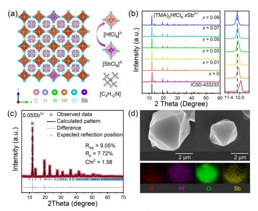
Fig. 1 (a) Schematic illustrations for the crystal structures of  $(TMA)_2HfCl_6$  and  $Sb^{3+}$  doping  $(TMA)_2HfCl_6$ . (b) XRD patterns of  $(TMA)_2HfCl_6$ :  $Sb^{3+}$  with different Sb3+ doping concentrations. (c) Rietveld refinement of XRD patterns for TMA2HfCl6. (d) Energy-dispersive spectrometer (EDS) mapping of corresponding elements Hf, Sb, and Cl in (TMA)<sub>2</sub>HfCl<sub>6</sub> and Sb<sup>3+</sup> hybrid.
