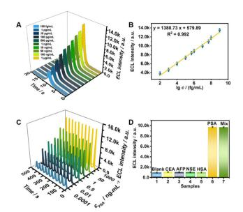
Fig. 4 (A) ECL intensity-potential profiles of the constructed CRE aptasensor with various concentrations of the target PSA (100 fg  $mL^{-1}\sim 1~\mu g$ mL<sup>-1</sup>). (B) Corresponding calibration plot of the constructed CRE aptasensor for PSA detection. (C) Stability of the constructed CRE aptasensor. (D) Selectivity of the constructed CRE aptasensor with relevant interfering molecules. Error bars = SD, (n = 3).
