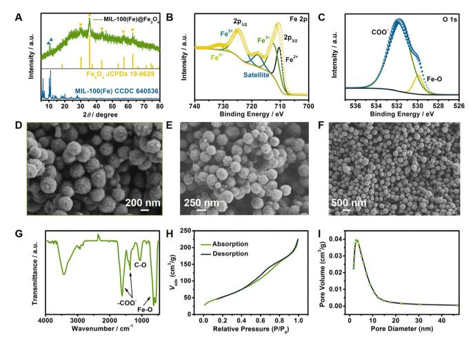
Fig. 2 (A) XRD pattern of as-synthesized MIL-100(Fe)@Fe<sub>3</sub>O<sub>4</sub>, and simulated patterns of Fe<sub>3</sub>O<sub>4</sub> and MIL-100(Fe). (B) Fe 2p and (C) O 1s XPS spectra. SEM images of (D) Fe<sub>3</sub>O<sub>4</sub> and (E and F) MIL-100(Fe)@Fe<sub>3</sub>O<sub>4</sub>. (G) FT-IR spectrum of as-prepared MIL-100(Fe)@Fe<sub>3</sub>O<sub>4</sub>. (H) Nitrogen adsorption-desorption isotherm and (I) pore-size distribution of MIL-100(Fe)@Fe<sub>3</sub>O<sub>4</sub>.
