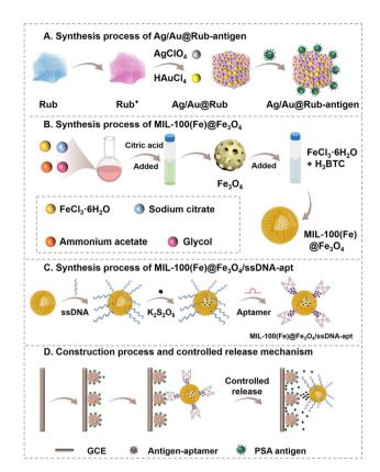
Scheme 1 Synthesis process of (A) Ag/Au@Rub-antigen, (B) MIL-100 (Fe)@Fe<sub>3</sub>O<sub>4</sub>, and (C) MIL-100(Fe)@Fe<sub>3</sub>O<sub>4</sub>/ssDNA-apt, and (D) the construction process and controlled release mechanism of the CRE aptasensor.
