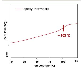
Fig. 4 DSC curve of an epoxy thermoset.
