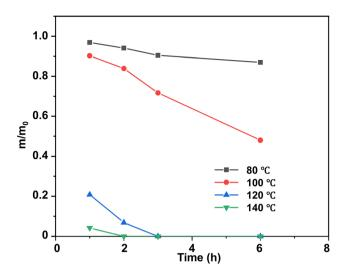
Fig. 5 Normalized residual mass of epoxy in DBU/EG solution at different temperatures as a function of time at 120 °C.
