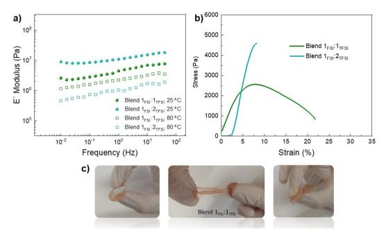
Fig. 4 DMTA frequency scan at 1% strain and at 25 and 80 °C (a); stress—strain curves at 25 °C for protic Blend  $1_{FSI}$ :  $1_{TFSI}$  and Blend  $1_{FSI}$ :  $2_{TFSI}$  at 25 °C and 75% RH (b); and pictures of Blend  $1_{FSI}$ :  $1_{TFSI}$  at 75% RH (c).
