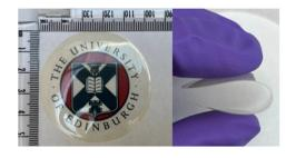
Fig. 4 A robust, optically clear, self-standing film of BTFMA-DPE fabricated from chloroform solution using the techniques of simple solventcasting (5 cm diameter, 100 um thick).
