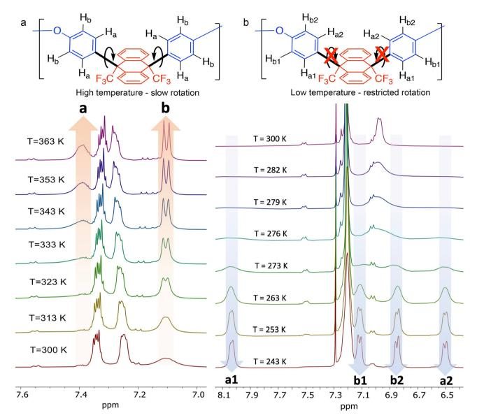
Fig. 3 Variable temperature NMR of polymer BTFMA-DPE acquired in the ranges (a) 300-363 K (in DMF-d<sub>7</sub>) and (b) 243-300 K (in CDCl<sub>3</sub>). Due to hindered rotation of the benzene rings of the DE monomeric unit, the peak for the hydrogens (H<sub>a</sub>) adjacent to the new bond only becomes distinct at higher temperatures. At lower temperatures, rotation is frozen so that each of the protons H<sub>a1</sub>, H<sub>a2</sub>, H<sub>b1</sub> and H<sub>b2</sub> show a distinct peak.
