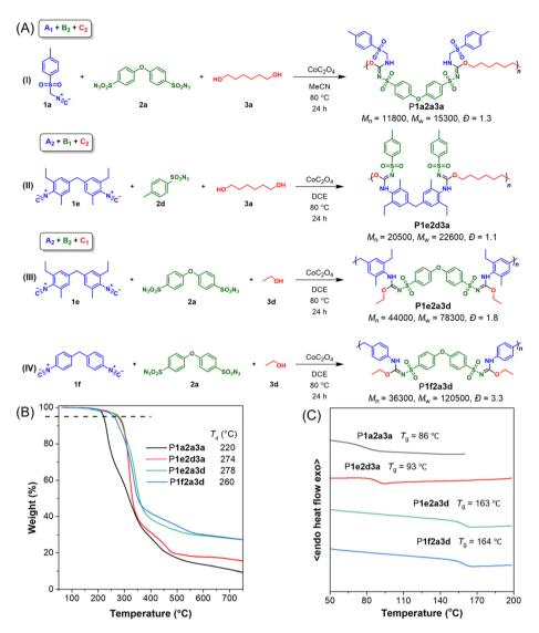
Fig. 4 (A) The specific structures and molecular weights of P1a2a3a, P1e2d3a, P1f2a3d and P1e2a3d. (B) TGA thermograms of polymers recorded under nitrogen at a heating rate of 10 °C min<sup>-1</sup>. (C) DSC thermograms of polymers recorded under nitrogen during the second heating cycle at a heating rate of 10 °C min<sup>-1</sup>.
