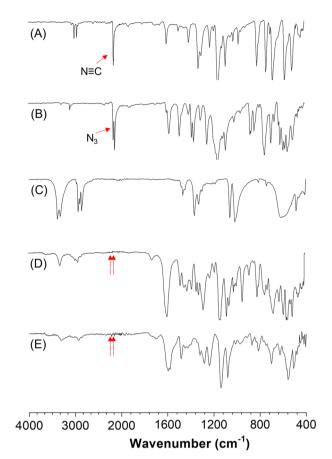
Fig. 1 IR spectra of (A) 1a, (B) 2a, (C) 3a, (D) model-1, and (E) P1a2a3a.
