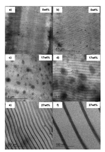
**Fig. 4** Transmission electron microscopy (TEM) images of thin slices from THF casting solution with respecting CoEtBAEMA content in weight percent (wt%): (a and b) PS<sub>797</sub>-b-(PCoEtBAEMA<sub>7</sub>-co-PMMA<sub>8</sub>), (cand d) PS<sub>773</sub>-b-(PCoEtBAEMA<sub>31</sub>-co-PMMA<sub>12</sub>), (e and f) PS<sub>773</sub>-b-(PCoEtBAEMA<sub>57</sub>-co-PMMA<sub>27</sub>).
