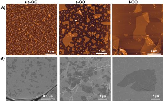
Fig. 1 Morphological characterization of us-GO, s-GO and I-GO. (A) Height atomic force microscopy (AFM) images. (B) Scanning electron microscopy (SEM) images.
