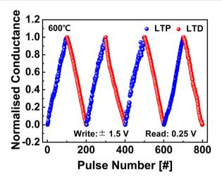
Fig. 10 Conductance saturation characteristics of HfO<sub>2</sub>/ZnO synaptic devices with thermal annealing at 600 °C under a series of positive pulses with different voltage amplitude.
