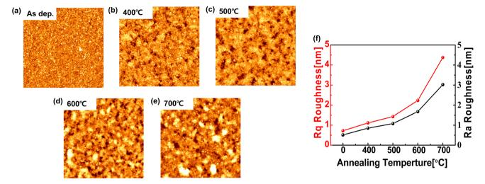
Fig. 2 AFM surface topography images of ZnO films in bilayer  $HfO_2/ZnO$  synaptic devices (a) without thermal annealing, (b) with thermal annealing at 400 °C, (c) 500 °C, (d) 600 °C, and (e) 700 °C. (f) Dependence of the root mean square ( $R_q$  or  $R_{rms}$ ) and average roughness ( $R_a$ ) of ZnO films on thermal annealing.
