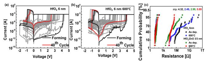
Fig. 7 Typical I-V switching behavior of 6 nm  $HfO_2$  (a) without and with thermal annealing (b) at 600 °C for 1 h in an  $N_2$  ambient compared with that of bilayer HfO<sub>2</sub>/ZnO synaptic devices under the same thermal annealing conditions. (c) Distribution and cumulative probability of the HRS and LRS of HfO<sub>2</sub> (6 nm) and bilayer 3 nm HfO<sub>2</sub>/3 nm ZnO synaptic devices without and with thermal annealing.
