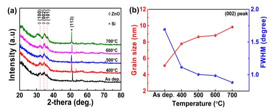
Fig. 3 (a) X-Ray diffraction spectra of  $HfO_2/ZnO$  films without and with thermal annealing from 400 °C to 700 °C. (b) Dependence of the full width at half maximum (FWHM) and average grain size of  $HfO_2/ZnO$  films on annealing temperature.
