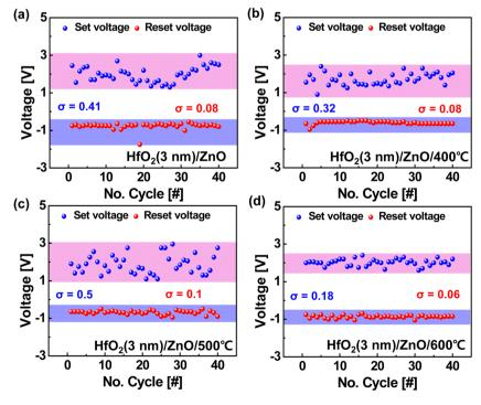
Fig. 6 Obtained VSET and VRESET distributions for 40 consecutive I-V sweeps for bilayer HfO<sub>2</sub>/ZnO synaptic devices (a) without and with thermal annealing at (b) 400 °C, (c) 500 °C, and (d) 600 °C.
