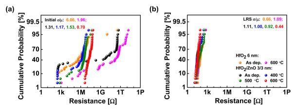
Fig. 4 Distribution and cumulative probability of (a) the initial state during the electroforming process and (b) the low-resistance state (LRS) for single-layer HfO2 and bilayer HfO2/ZnO synaptic devices without and with thermal annealing, where the initial state and LRS were extracted at a read voltage of  $\pm 0.3$  V.
