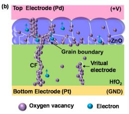
Fig. 11 Schematic illustration of the transition mechanism during the conductive filamentary formation in bilayer HfO<sub>2</sub>/ZnO synaptic devices (a) without and (b) with thermal annealing. Crystallized ZnO films formed by thermal annealing between the top Pd electrode and the HfO2 layer remarkably improve  $O^{2-}$  migration from the HfO<sub>2</sub> layer to the ZnO bulk and the top electrode interface.
