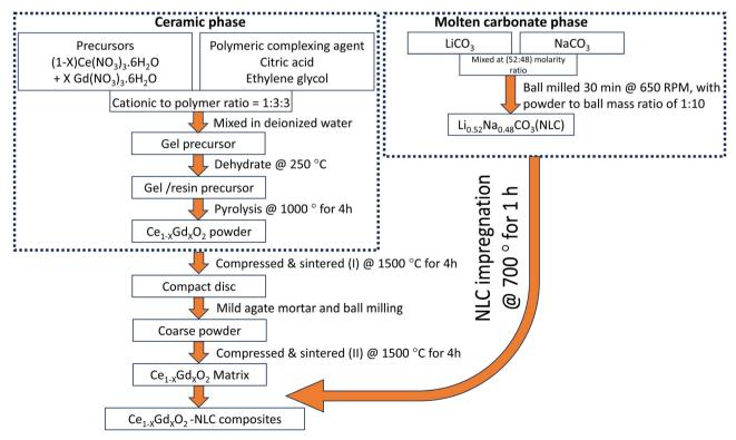
Fig. 1 Flow chart of synthesis of  $Ce_{1-X}Gd_XO_2$ -NLC composites membrane.
