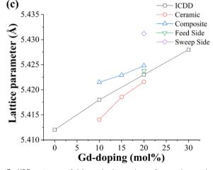
Fig. 3 XRD patterns of (a) crushed powders of ceramic matrices of increasing Gd-doping of 10 mol%, 15 mol%, and 20 mol% and (b) relevant composites after impregnation of NLC at 700 °C for 1 h, and (c) lattice parameter evaluated for ceramic phase at various situations. Enlarged views of prinicipal reflections are shown on the right-hand side of the main pattern
