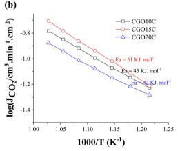
Fig. 6 Temperature-dependent (a)  $CO_2$ -separation flux, and (b) Arrhenius behaviour of CGO10C, CGO15C, and CGO20C composite membranes.
