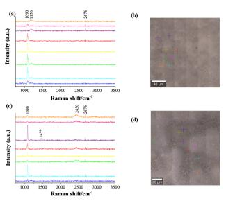
Fig. 8 FT-Raman spectra across selected places on the feed (a) and sweep (c) sides of the CGO20C composite membrane, with respective optical images of scanned areas (b) and (d). The colours of the crosses and spectra relate the analysis point to the signal from the corresponding spot.
