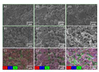
Fig. 4 SEM micrographs of CGO10, CGO15, and CGO20 matrices are represented by A1, A2, and A3 in the first row, while the correpsonding SEM and EDS mapping of composites are represented as B1, B2, and B3, and C1, C2, and C3 in the second and third rows of the figure, respectively.
