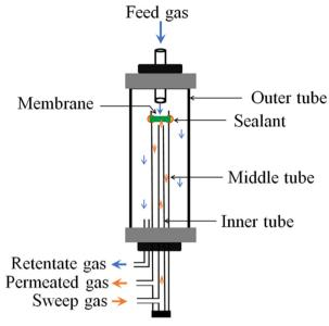
Fig. 2 Schematic of laboratory-built CO<sub>2</sub>-separation setup.
