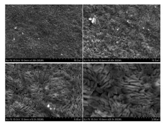
SEM images of the sweep side of the CGO20C membrane cap tured after a CO<sub>2</sub>-separation test at different magnifications.
