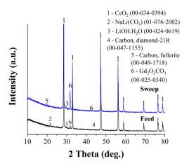
Fig. 7  $\,$  X-ray analysis performed on the feed and sweep sides of CGO20C after CO<sub>2</sub>-separation.
