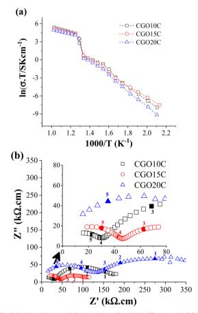
Fig. 5 (a) Arrhenius and (b) impedance (at 250 °C) plots of CGO10C, CGO15C, and CGO20C composite membranes. 1, 2, 3, 4, and 5 are data acquisition points obtained at sweep frequencies of 112 Hz, 790 Hz, 2.8 kHz, 96 kHz, and 500 kHz, respectively.
