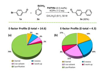
Fig. 2 E-Factor profile for the model SM reaction between 1a and 2a before (a) and after (b) the recovery of H<sub>2</sub>O used in product purification.
