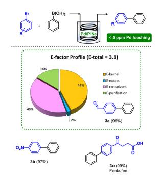
Fig. 3 Continuous flow SM coupling between 1 and 2a and the E-factor profile for the synthesis of the product 3a.
