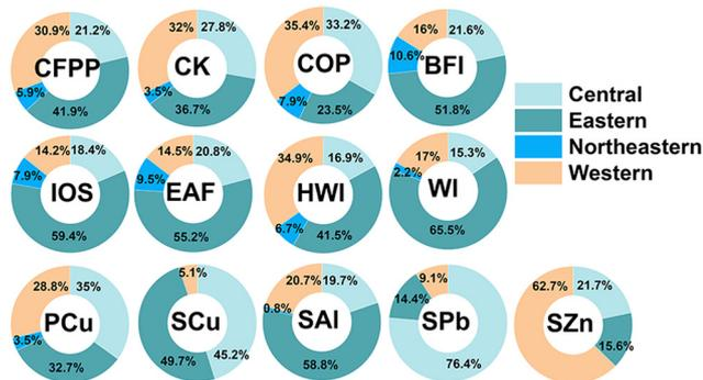
**Fig. 5** Proportions of Ti-containing NP emissions by industrial source in the four economic regions of China. PCu = primary copper smelting; SCu = secondary copper smelting; SAI = secondary aluminum smelting; SPb = secondary lead smelting; WI = municipal solid waste incineration; CK = cement kiln co-processing of solid waste; IOS = iron-ore sintering; COP = coking plant; HWI = hazardous-waste incineration; CFPP = coal-fired power plant; BFI = blast-furnace pig iron steelmaking.
